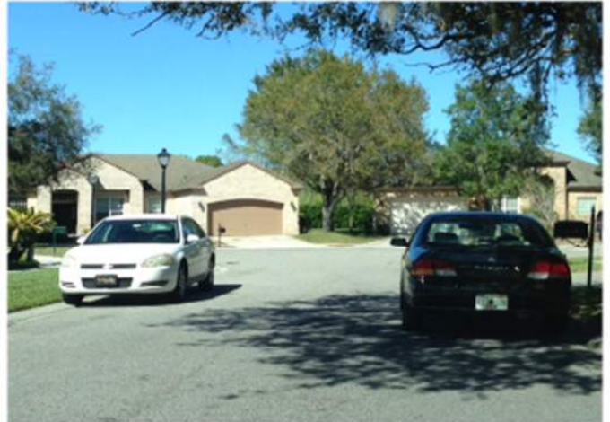
No parking directly opposite another vehicle where this action could create a choke point for safe emergency vehicle access.
