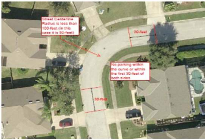
No parking within 30' of or in any curve with a centerline street radius of 100' or less as determined by engineers.
